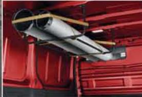
An interior roof rack provides useful extra load carrying capacity.
