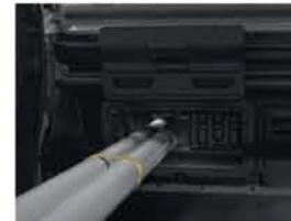
Bulkhead flap lifts to allow extra long objects - up to 3.75M in the L1 NV300 or 4.15M in the L2 NV300.
