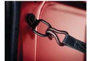
Up to 18 built-in side and floor mounted tie-downs to keep your load secure.
