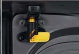
This clever device lets you lock a rear door open and enables you to carry longer loads safely (starting from E1).
