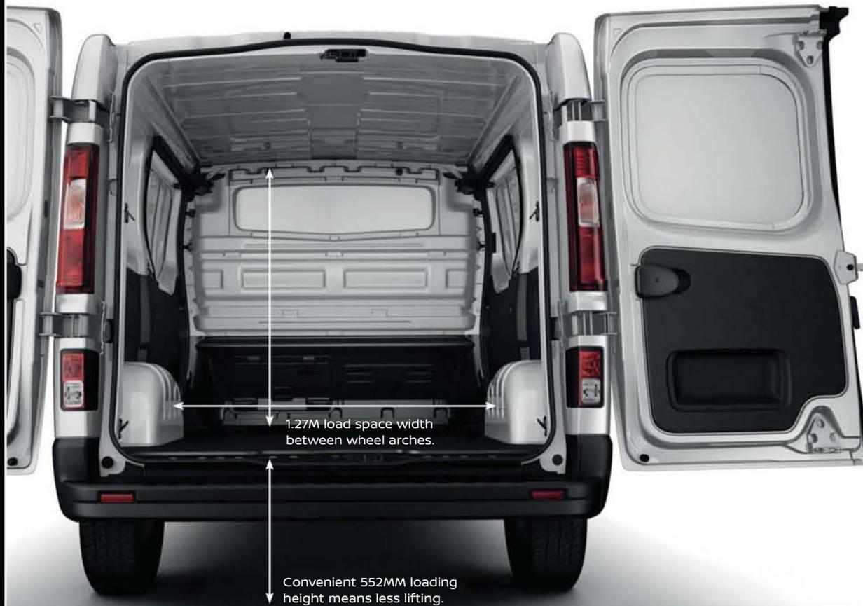
1.27M load space width between wheel arches.
